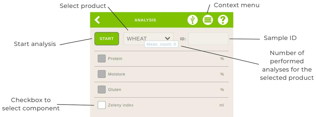
Components can be turned off by unchecking the checkbox:
