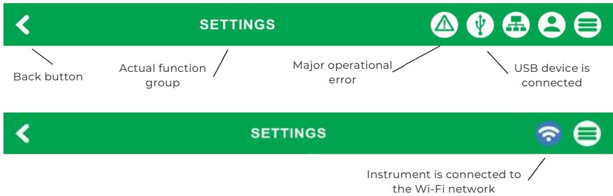
In an everyday use, for a normal user there are only 2 icons displayed on the status bar, if the instrument is not connected to the internet and no USB-device is connected:
