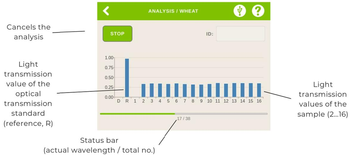
At the end of the measurement the results are displayed on the screen:
