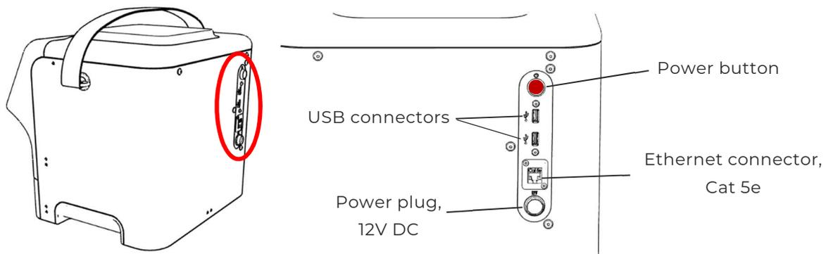
Connect the instrument to the electric network (100~240VAC, 50/60Hz) and switch it on with the red button found on the back of the instrument.
