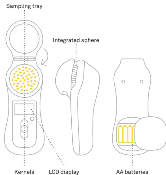
The technical principle is **Near-infrared (NIR) spectroscopy** in the so-called third overtone wavelength range. This technique has been used in laboratory instruments for years. Field Lab is the first to realize such an instrument in a handheld format.
