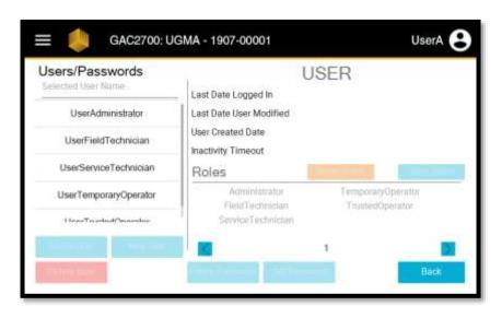
The GAC<sup>®</sup> 2700 can be configured for multiple levels of user interaction with the settings that would affect metrology of the instrument. This menu provides the Admin with the ability to configure what pre-defined set of permissions a user would have in the form of roles.
