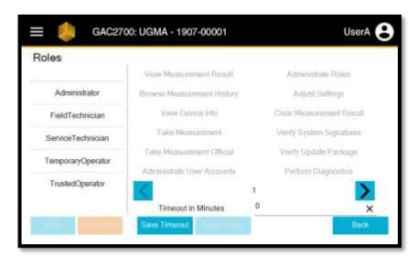
The GAC<sup>®</sup> 2700 can create preset lists of permissions which are called 'Roles'. These sets of permissions will allow the admin to define whether a specific operator is able to only conduct a moisture measurement, adjust settings, download new software, all of these, none of these, or conduct other interactions with the GAC<sup>®</sup> 2700.
