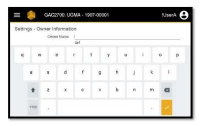
The GAC<sup>®</sup> 2700 permits the user to apply owner information into the instrument memory in order to aid with asset tracking.
